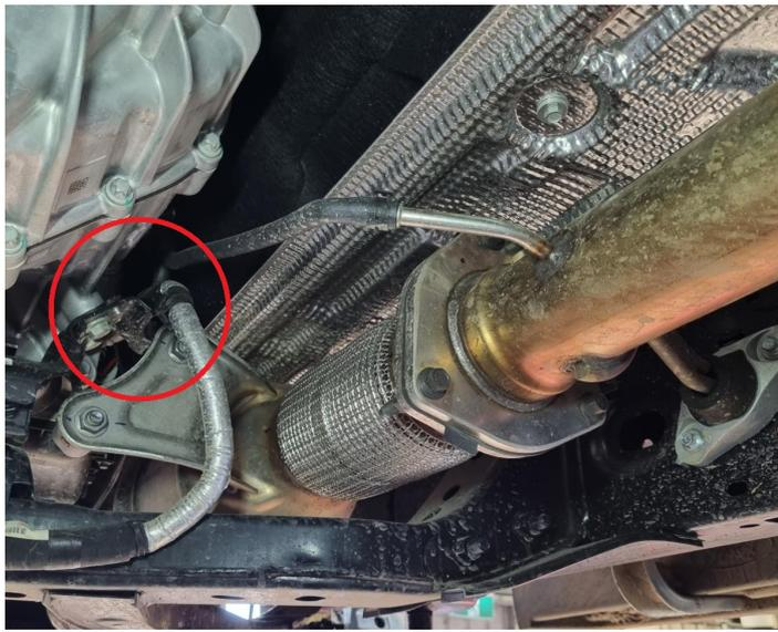
1. Locate factory exhaust pressure sensor on side of transmission, beside DPF.
